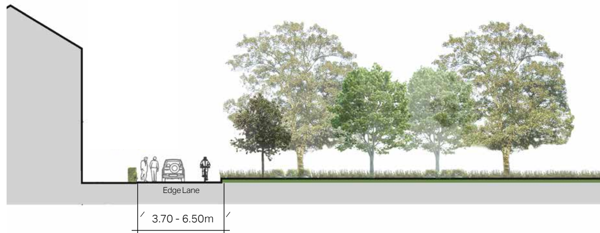
Figure 45: Diagram of a suitable edge lane used at the edge of the village to act as a transition into the countryside.
